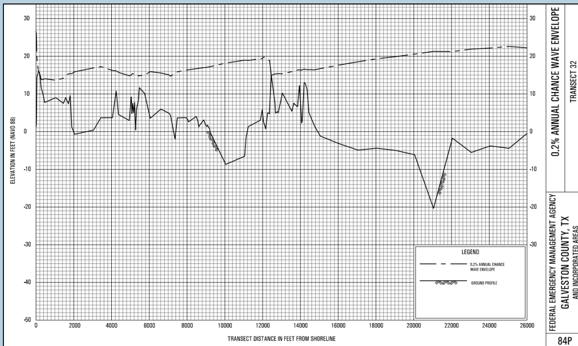
Figure 12. Example of a coastal transect profile with 0.2% annual-chance wave envelope elevations
